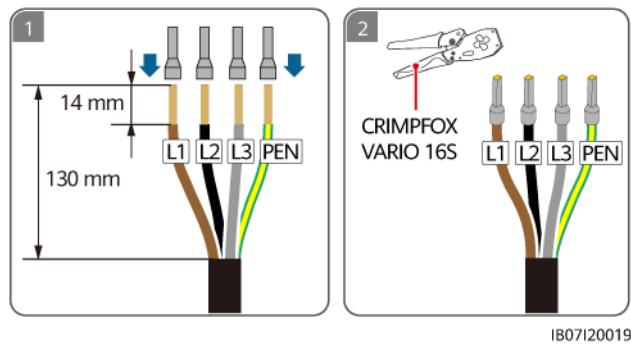
**Step 2** Connect the output power cable to the backup load. Check the load to be connected based on the backup load requirements.
