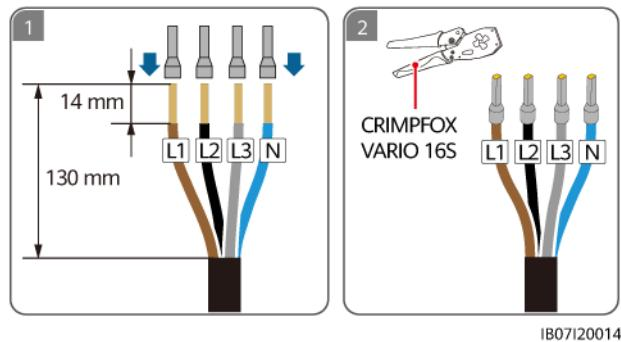
**Figure 5-17** Crimping AC cord end terminals (TN-C system)
