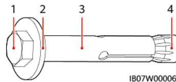
(1) Hexagonal bolt      (2) Flat washer      (3) Sleeve      (4) Conical nut
