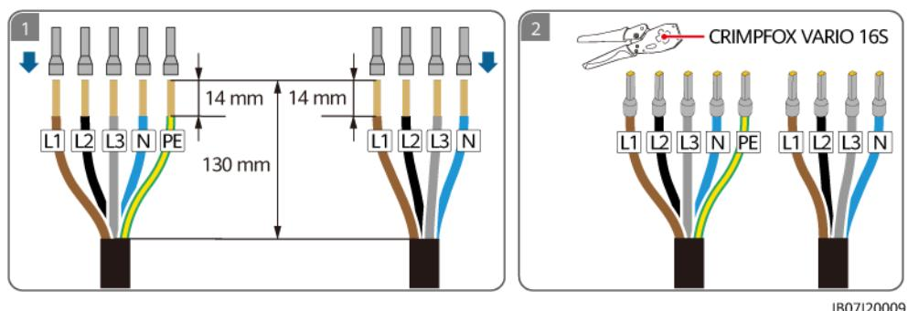
**Figure 5-9** Crimping AC cord end terminals (TN-C system)
