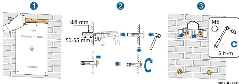
**Step 3** Install the SmartGuard on the mounting bracket and tighten the nuts.
