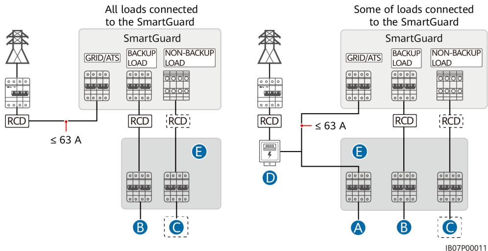
(A) Load not connected to the SmartGuard      (B) Backup load      (C) Non-backup load
