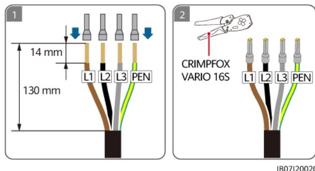
**Step 2** Connect the non-backup load output power cable.
