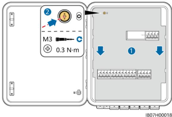
**Step 2** Before closing the maintenance compartment door, turn on the four switches shown in the following figure (using the connection to three parallel MAP0 inverters as an example).
