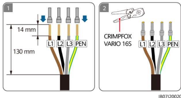
**Step 3** Connect the grid AC output power cable.
