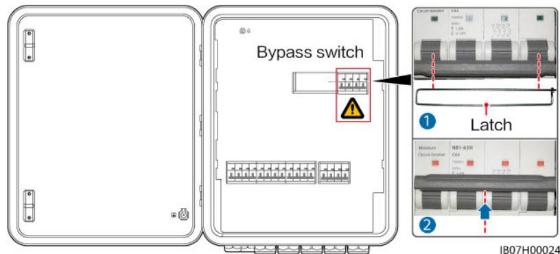
**Step 3** Turn on the four switches shown in the following figure (using the connection to three parallel MAP0 inverters as an example).
