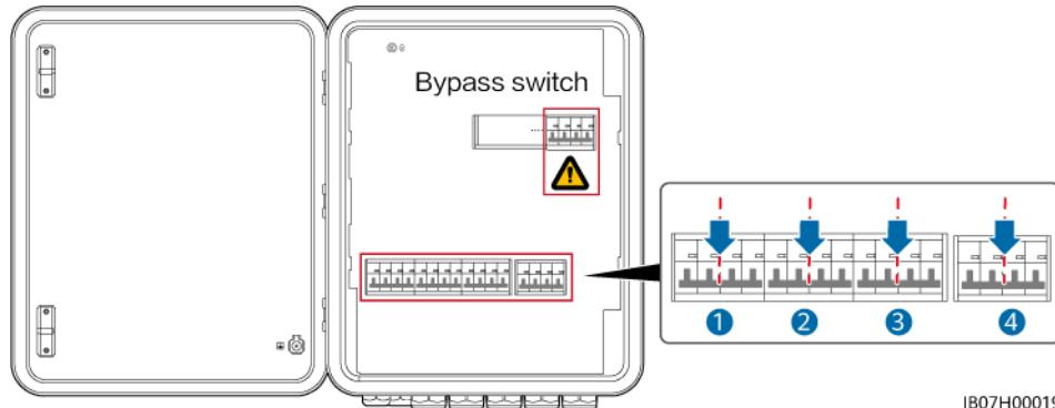
2. Remove the bypass switch latch, turn on the bypass switch, and then turn on switches ③ and ④ shown in the figure.
