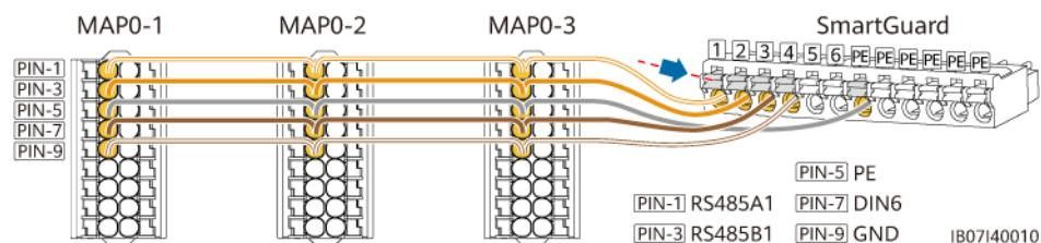
**Step 3** Connect the signal cables of the SmartGuard.
