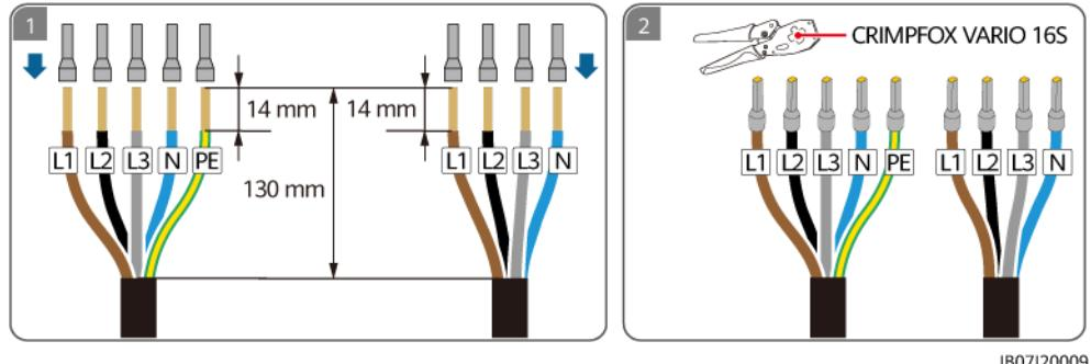
**Figure 5-22** Crimping AC cord end terminals (TN-C system)
