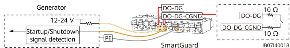
**Figure E-2** Generator alarm signal
