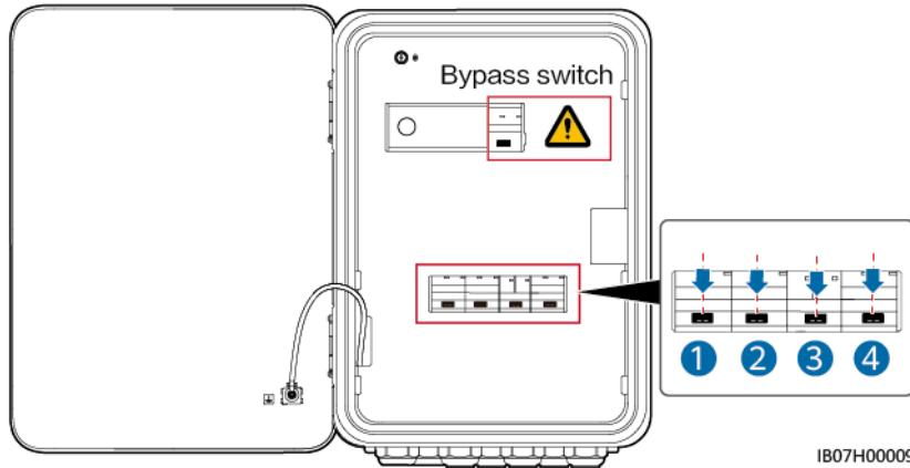
2. Remove the bypass switch latch, turn on the bypass switch, and then turn on switches ① and ④ shown in the figure.
