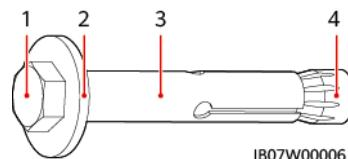
(1) Hexagonal bolt      (2) Flat washer      (3) Sleeve      (4) Conical nut
