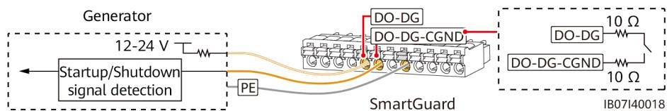
**Figure E-2 Generator alarm signal**
