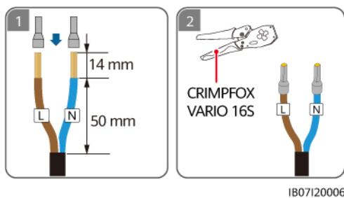
**Step 2** Connect the backup load output power cable.
