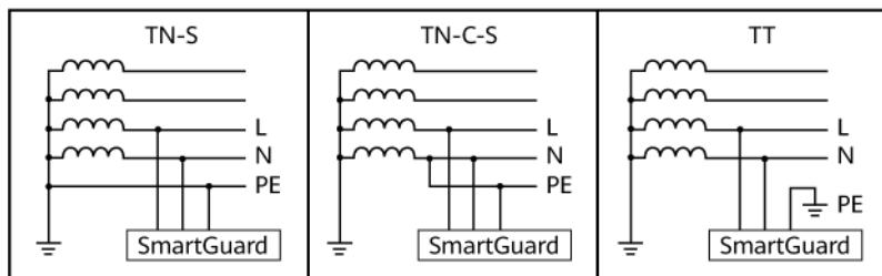
Figure 2-8 Earthing system (L1/L2 dual-live-wire connection)
