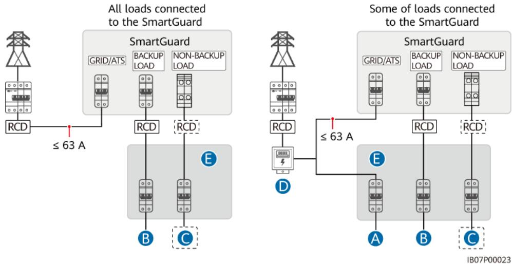
(A) Load not connected to the SmartGuard
