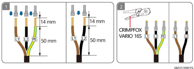
**Step 2** Connect the non-backup load output power cable.
