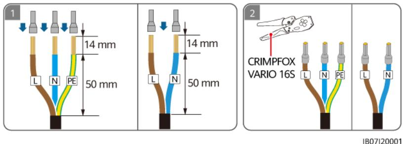
**Figure 5-22** Crimping AC cord end terminals (L1/L2 dual-live-wire connection)
