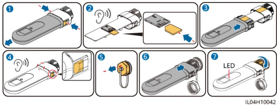
**Figure 5-44** Installing anti-theft components for the Smart Dongle
