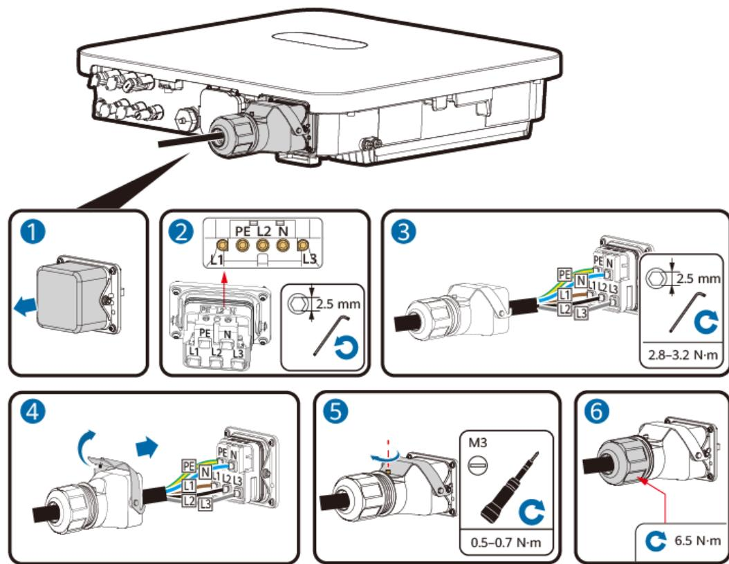
**Step 3** Check the route of the AC output power cable.
