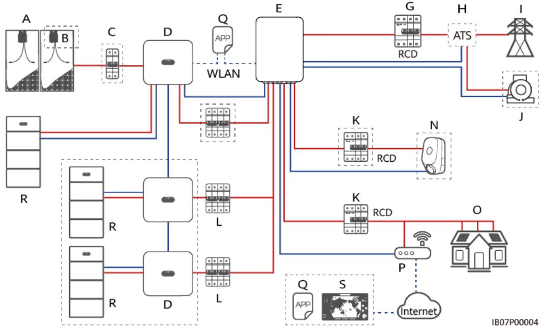
**Figure 2-5** Networking with some of loads connected to the SmartGuard (dashed boxes indicate optional components)
