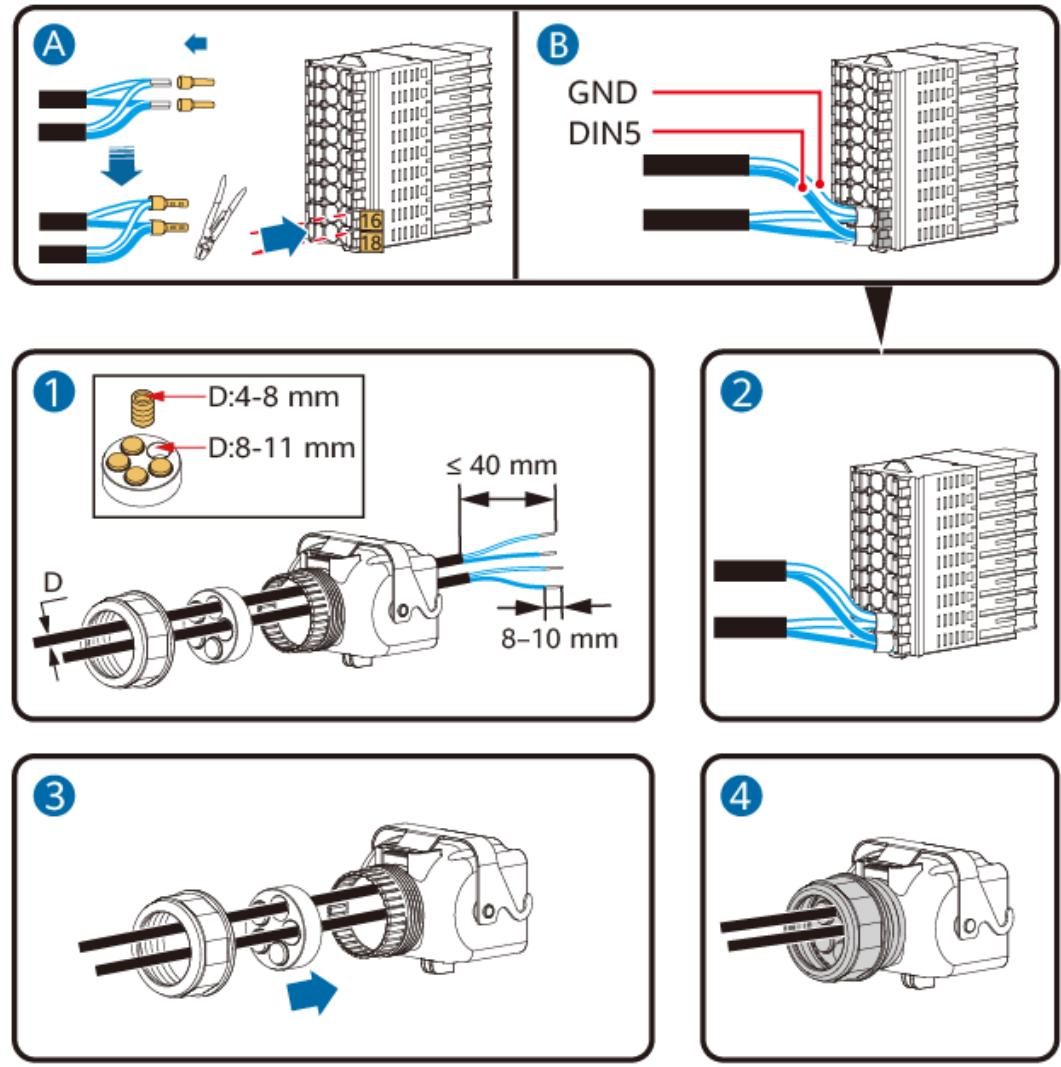
**Step 2** Connect the signal cable connector to the COM port.
