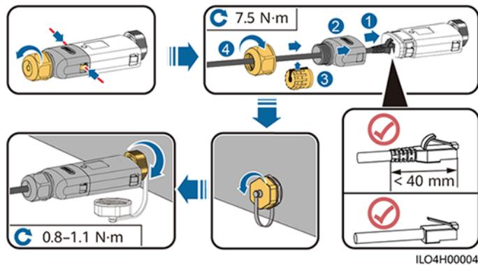
**Figure 5-42** Installing anti-theft components for the Smart Dongle
