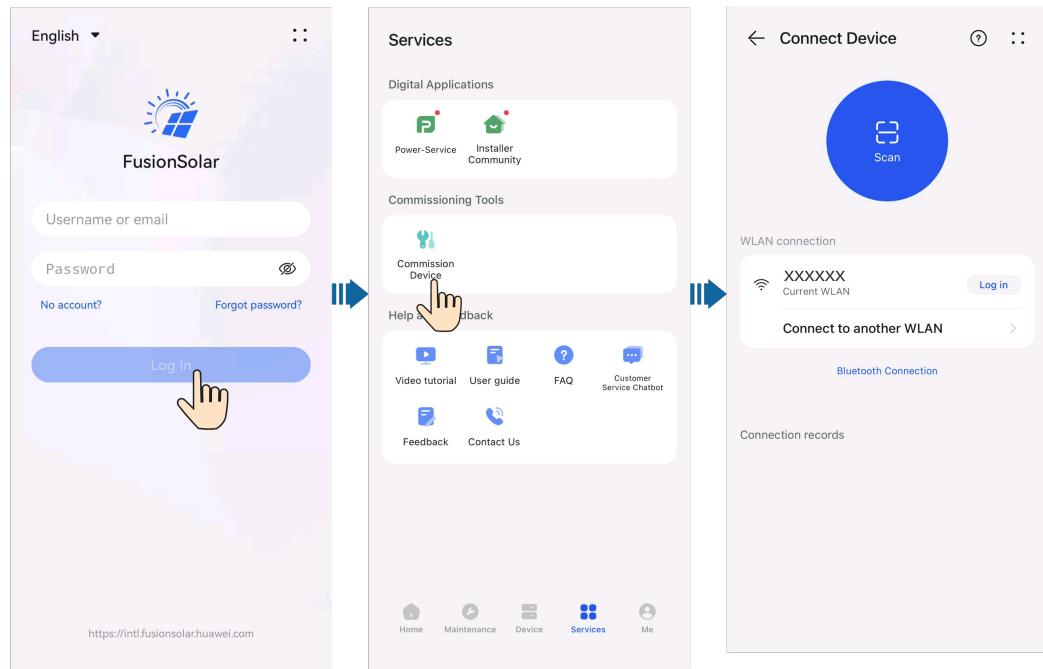
**Step 2** Connect to the solar inverter WLAN and log in to the device commissioning screen as the **installer** user.
