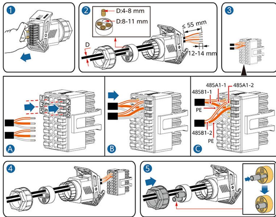
**Step 2** Connect the signal cable connectors to the COM port.
