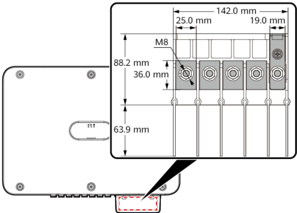
**Figure 5-5** Specifications of the crimped OT/DT terminal
