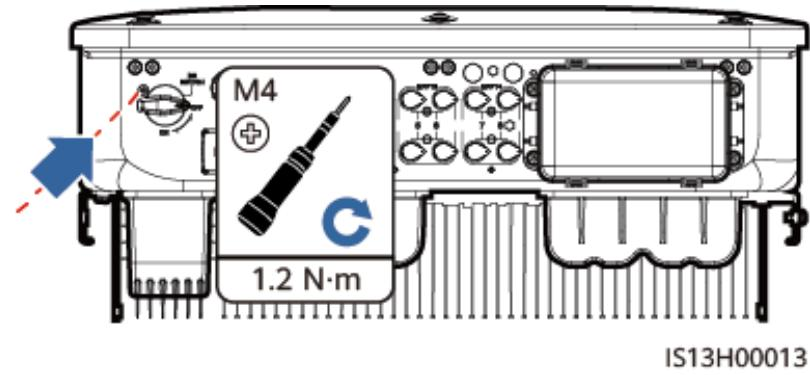
**Step 5** Turn off the DC switch (if any) between the inverter and PV strings.
