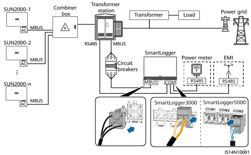
Figure 5-34 MBUS communication (C&I scenario in China)
