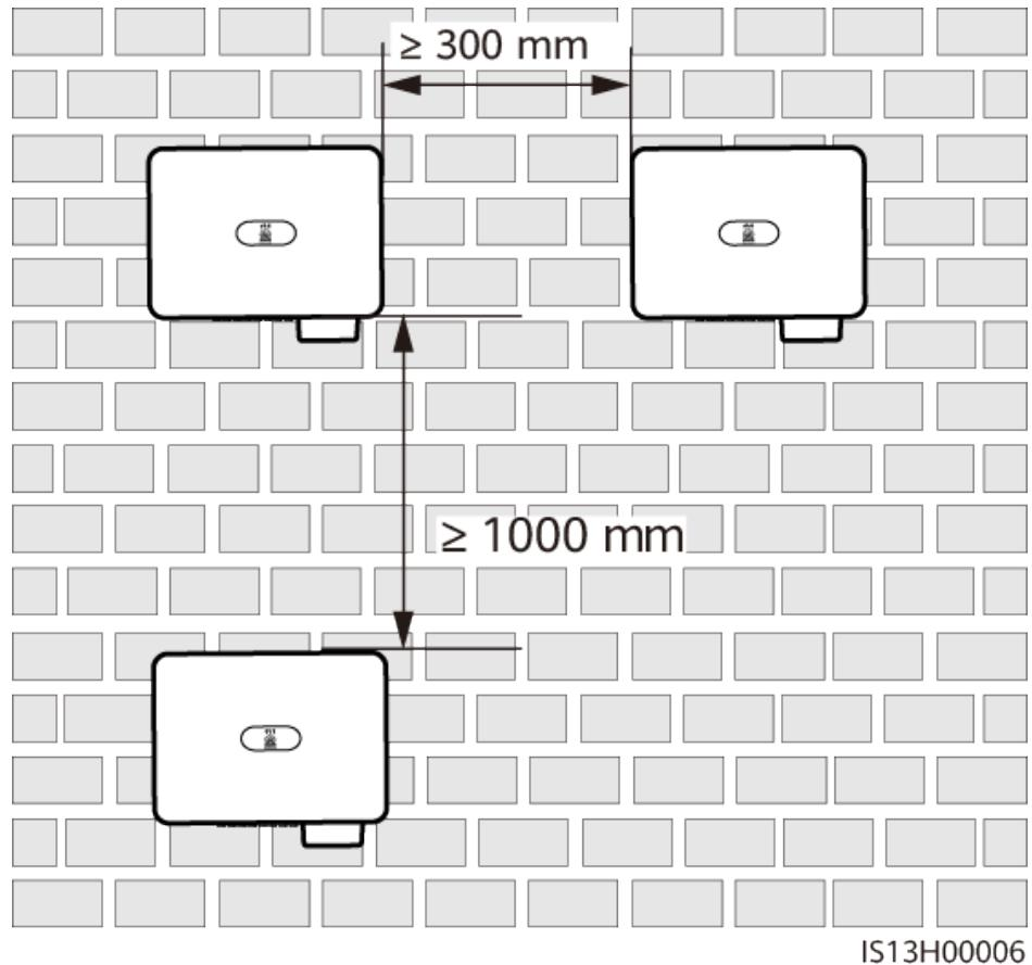
**Figure 4-7** Back-to-back installation mode (not recommended)
