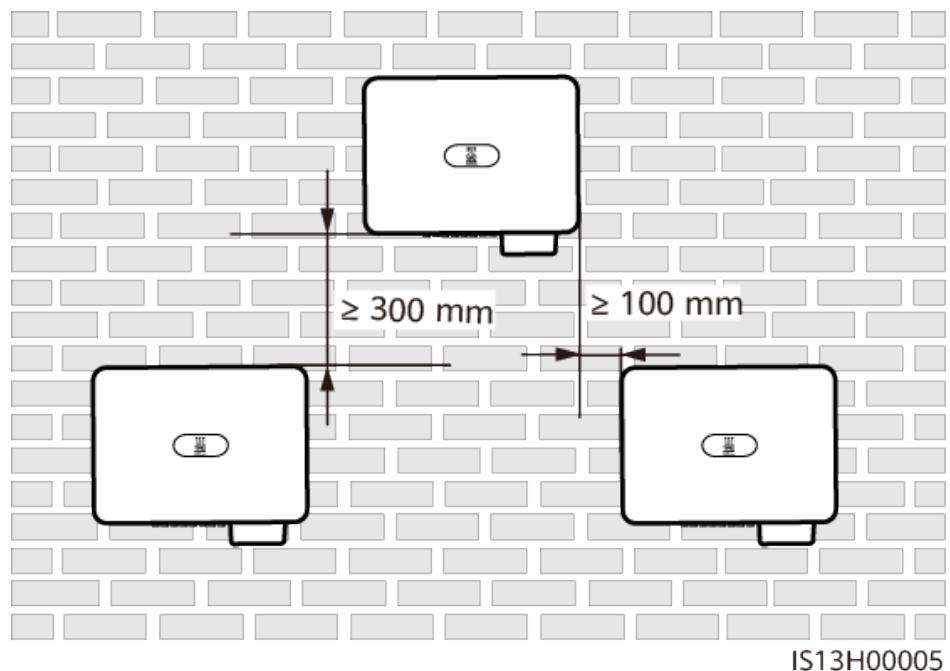
**Figure 4-5** Three-layer triangle installation mode (not recommended)
