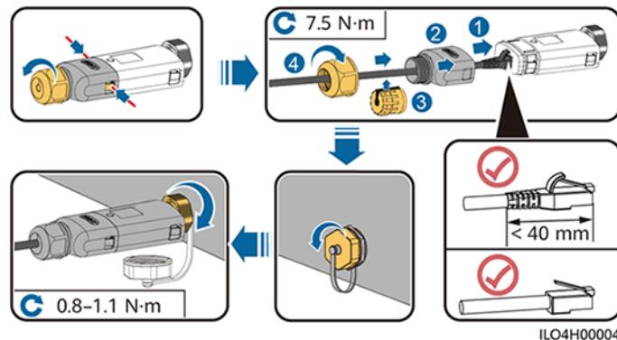
**Figure 5-17** Installing anti-theft components for the Smart Dongle
