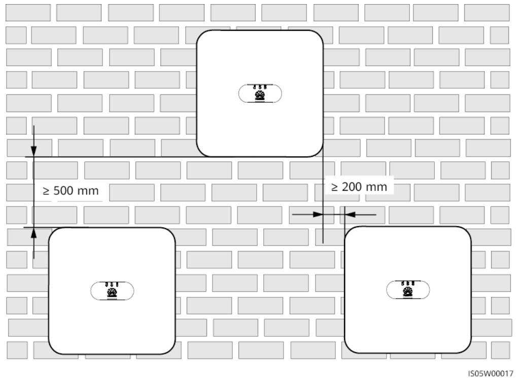
**Figure 4-5** Stacked installation (not recommended)
