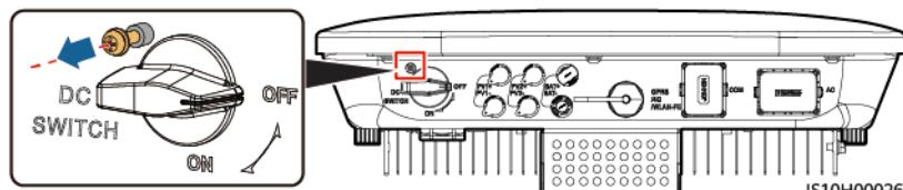
**Step 4** Turn on the DC switch (if any) between the PV string and the SUN2000.
