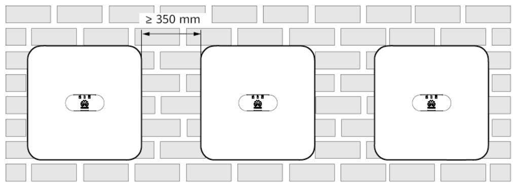
**Figure 4-4** Staggered installation (recommended)
