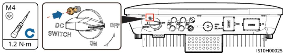
**Step 4** If there is a DC switch between the inverter and PV string, turn off the DC switch.
