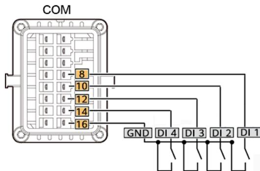
**Figure 5-41** Cable connections (SmartLogger networking)
