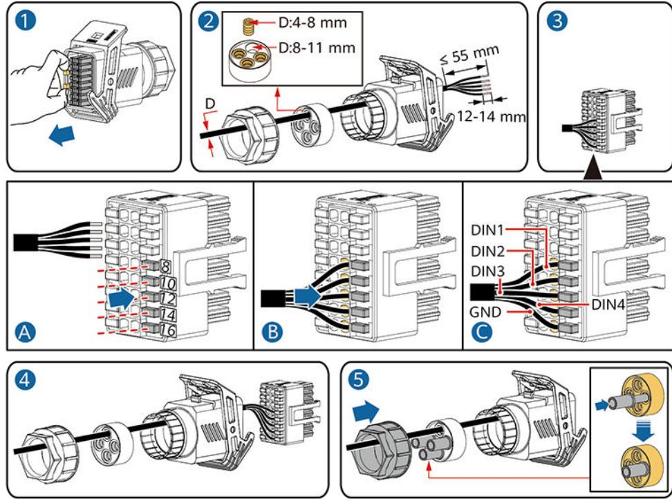
**Step 2** Connect the signal cable connector to the COM port.
