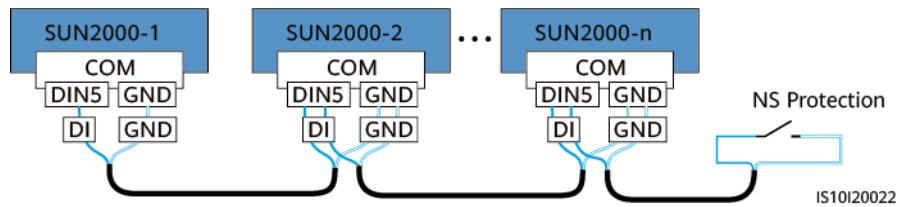
**Step 1** Connect the signal cables of the cascaded inverters to the signal cable connectors.
