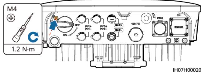
**Step 5** Turn off the DC switch between the inverter and PV strings.
