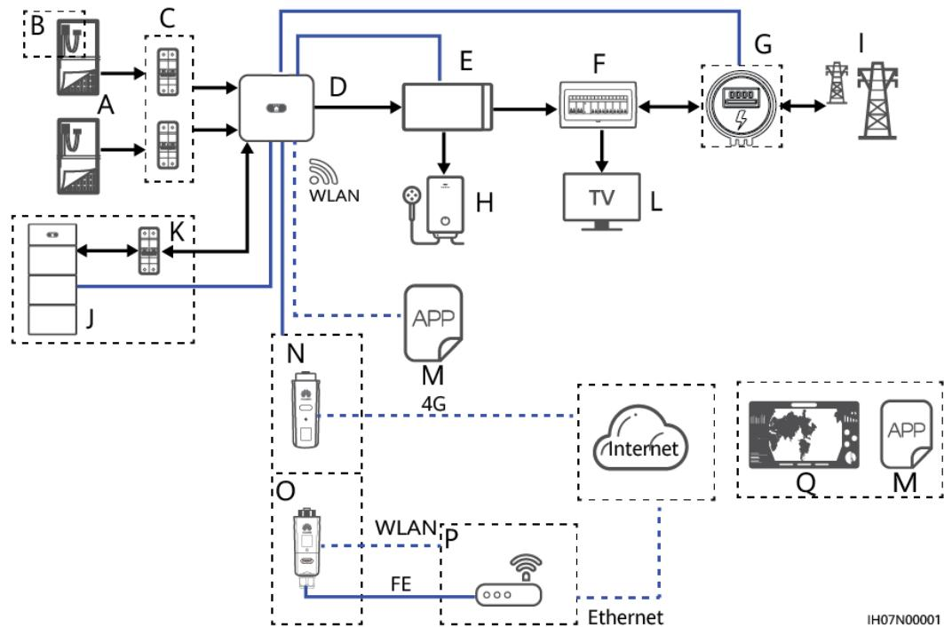
**Figure 2-3** Inverter cascading scenario (the components in dashed boxes are optional)
