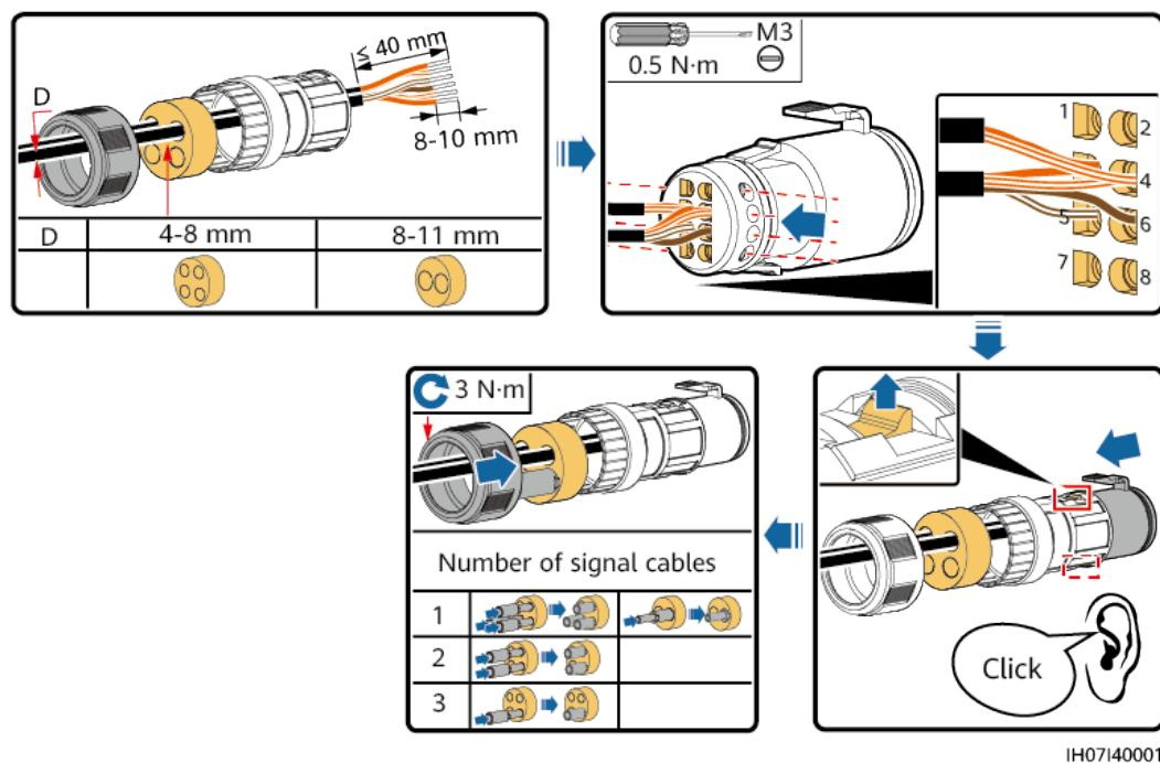
Figure 5-28 Assembling a signal connector (inverter cascading)
