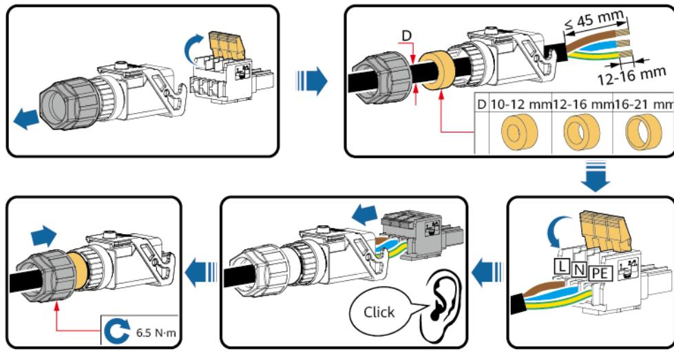
Figure 5-8 Assembling an AC connector (two-core wire)
