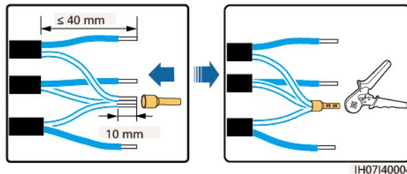
**Figure 5-27** Assembling a signal connector (single inverter)
