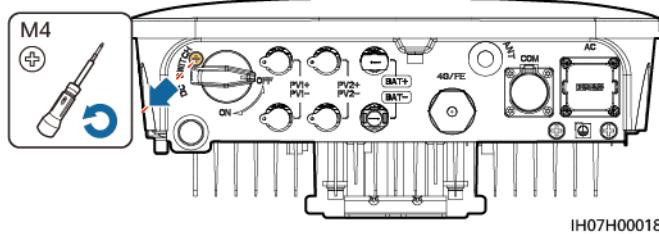
**Step 4** Turn on the DC switch between the PV string and the inverter if there is any.
