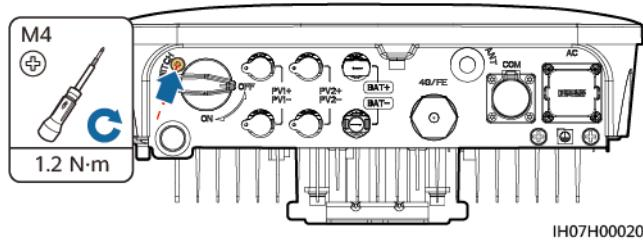
**Step 4** Install the inverter on the mounting bracket.
