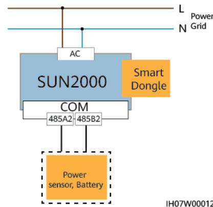
**Figure 5-20** Connecting cables to the power meter (single inverter)
