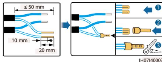
**Figure 5-26** Crimping three signal cables
