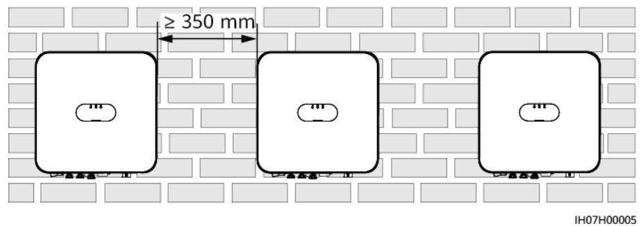
**Figure 4-4** Triangle installation mode (recommended)
