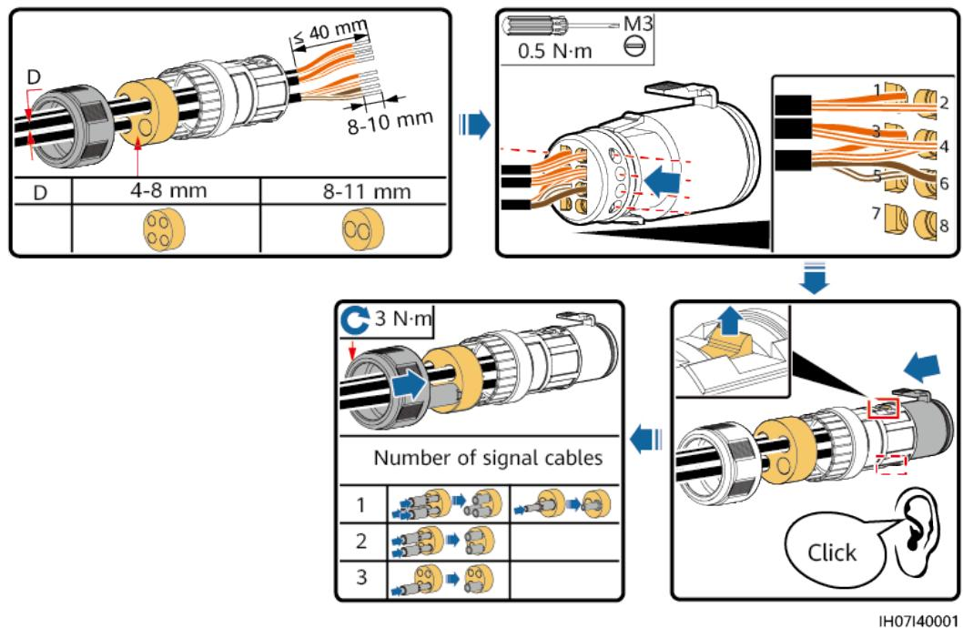
**Step 2** Connect the signal connector to the corresponding port.
