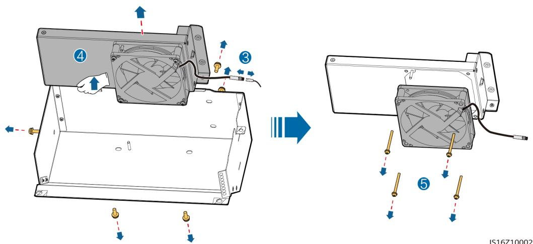
**Step 4** Install a new fan, install the fan bracket, bind the cable, and install the fan cover.
