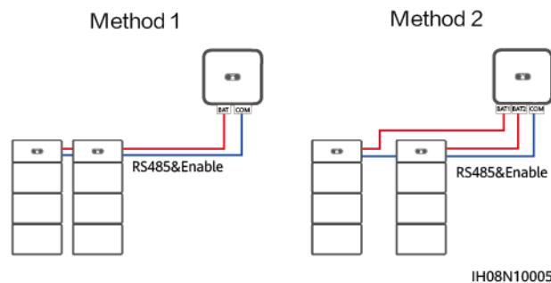
To connect the inverter to four batteries, refer to the following figure.
