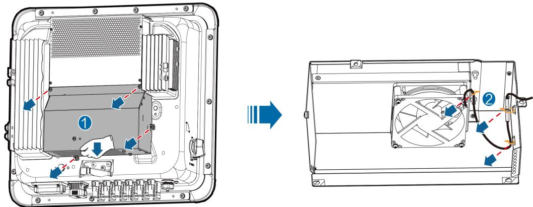
**Step 3** Disconnect the fan cable, take out the fan bracket, and remove the faulty fan.
