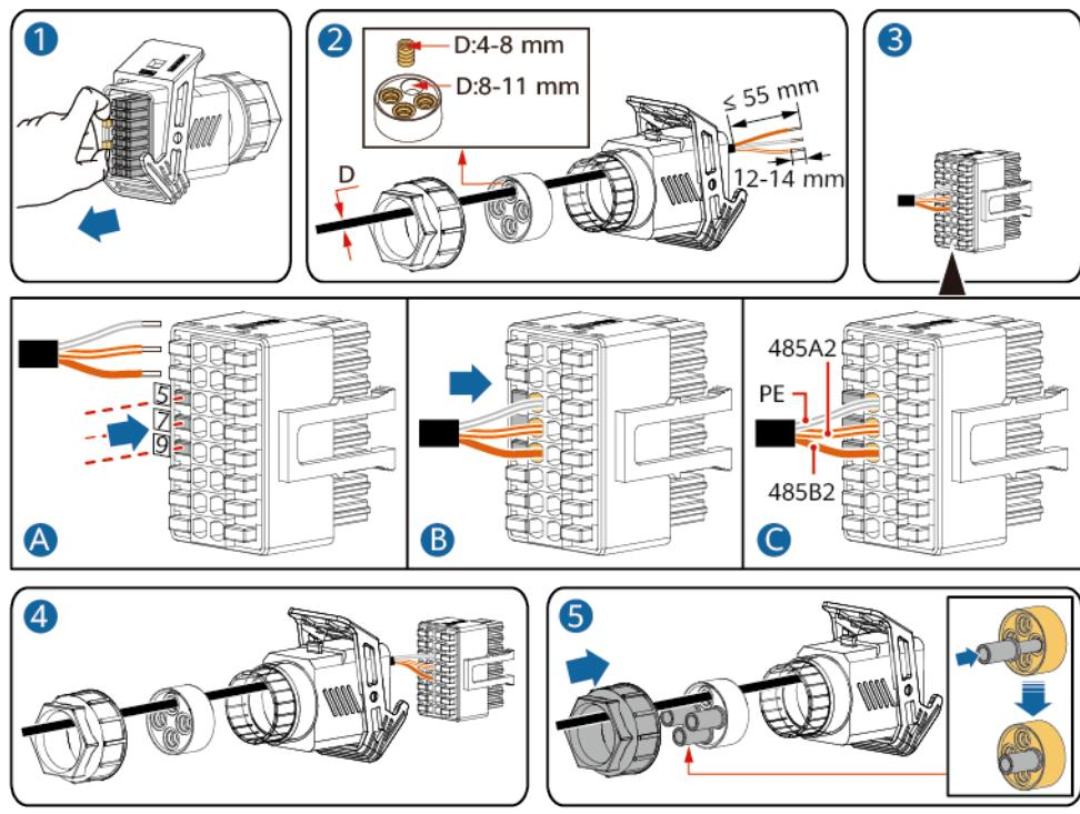
**Step 2** Connect the signal cable to the COM port.
