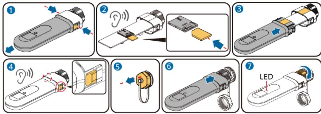
Figure 5-49 Installing anti-theft components for the Smart Dongle
