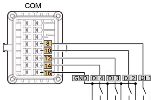
**Figure 5-39** Cable connections (SmartLogger networking)
