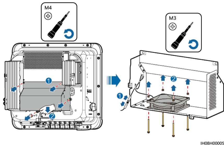
**Step 3** Install a new fan, connect and bind the cable, and install the fan cover.
