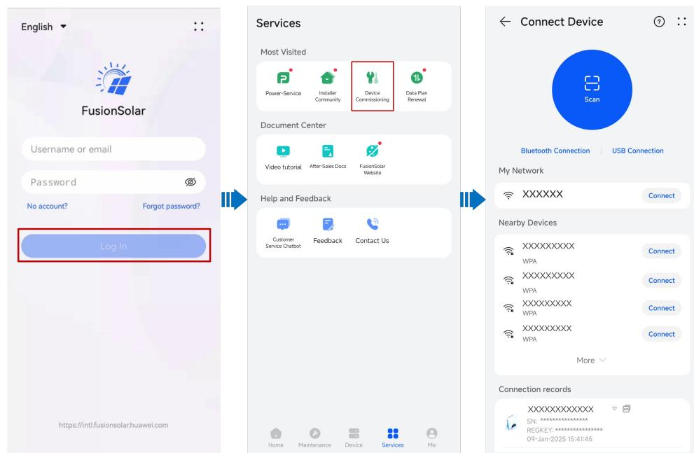
**Figure D-2** Method 2: mobile phone not connected to the Internet
