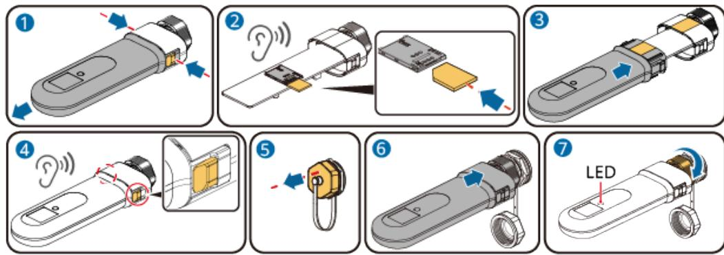
Figure 5-38 Installing anti-theft components for the Smart Dongle
