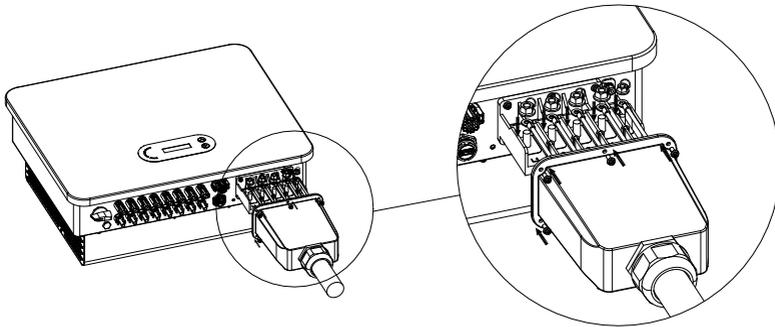
Figure 4-9 AC cable connection instruction diagram (2)
