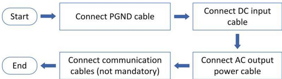
Figure 4-1 flowchart for connecting cables to the inverter
