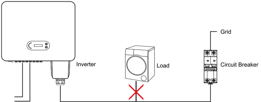
Figure 4-5 Incorrect connection between load and inverter
