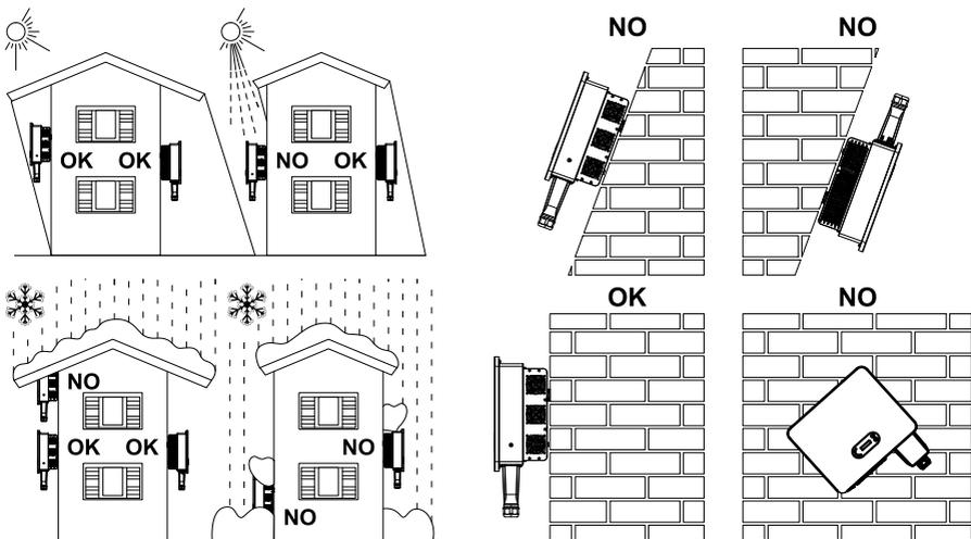
Figure 3-1 Installation Position Selection
