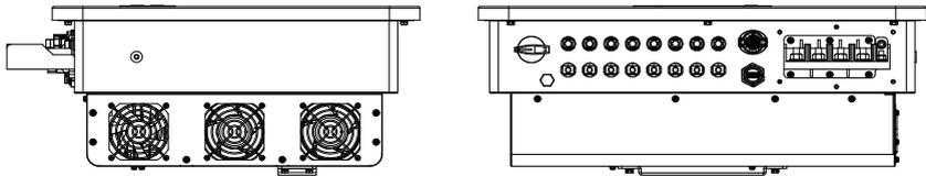
Figure 2-4 Bottom view (take 50KW for example)
