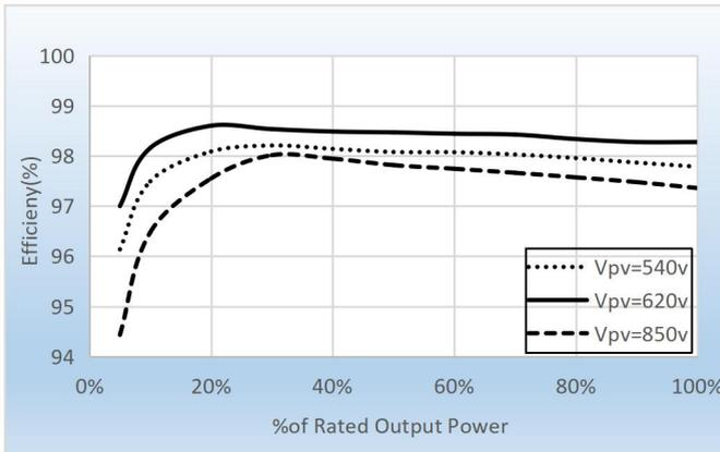
Figure 2-9 Power efficiency curve (take 50KW for example)
