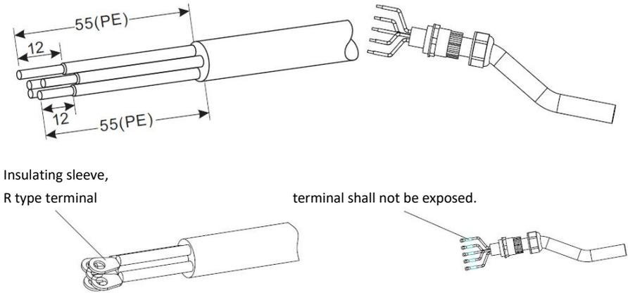
Figure 4-8 AC cable connection instruction diagram (1)
